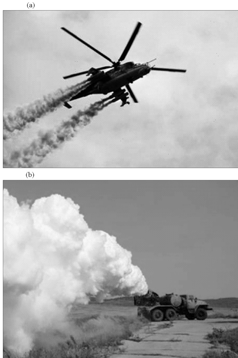
Fig. 1. Aerosol generators installed (a) on the helicopter and (b) on the car chassis.
