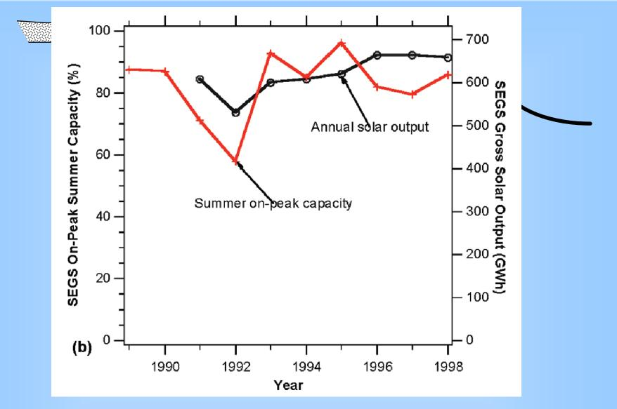
Output of solar electric generating systems (SEGS) solar thermal power plants in California (9 with a combined capacity of 354 peak MW). (Murphy, 2009, ES&T)
