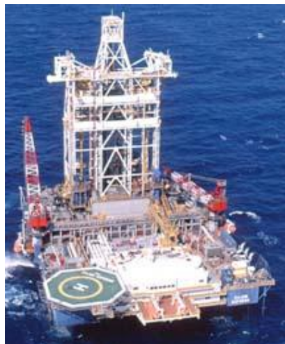
Figure 38: The Cajun Express deep water drilling rig. At 106x70m and with up to 10.6 km (35kft) of pipe down to a pocket of high pressure oil and natural gas, these off shore rigs are analogous to a floating geoengineering platform (Transocean image, http://www.deepwater.com/fw/main/Cajun-Express-52C17.html ).
